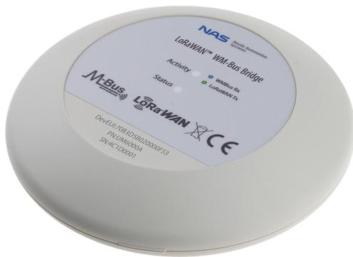
LoRaWAN™ WM-Bus Bridge is designed for receiving wireless M-Bus signals from utility meters and forwarding them via LoRaWAN networks to the service provider.
