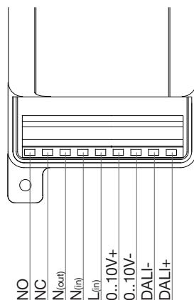
Pinout is also marked on the controller
