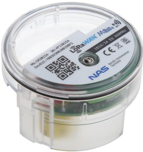
LoRaWAN® Modularis Module enables the acquisition of water consumption data and transmits it wirelessly to the available LoRaWAN® network or as a drive-by target in wM-Bus C1 or T1 mode.
